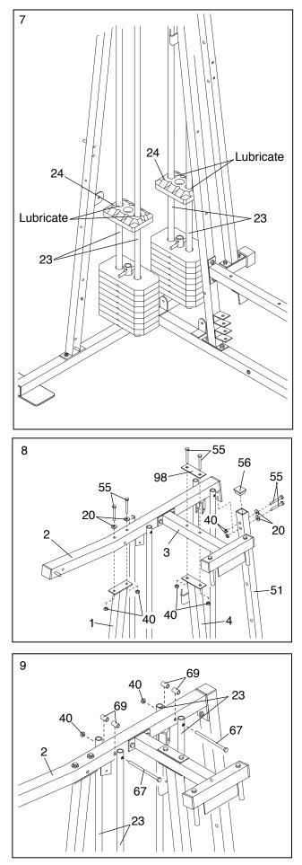
10. Press a 2" Square Inner Cap (56) into each end of the Leg Press Arm (9).
